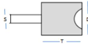
**TIPO A-38****D= 25 mm****T= 25.4 mm****S= 6.4 mm**
